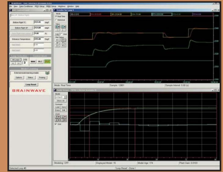
In addition to delivering consistent glass to bushings, model based control feeds forehearth temperatures forward to allow bushings to be prepared for incoming temperatures and adapt to them more effectively than PID loops. This helps bushings overcome deficiencies in forehearth temperature.
