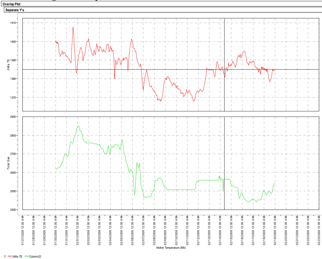
Figure 3: Temperature and Gas Flow before and after Model Based Control
